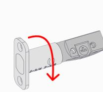
If the T-shaped hole is centered in the door hole, no adjustment needed. Proceed to the next step. If the T-shaped hole is NOT centered in the door hole, adjust needed. See "Bolt adjustment"
