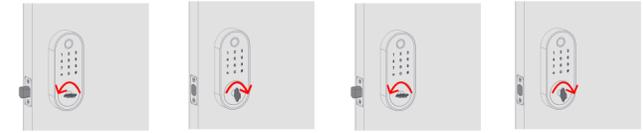
Ensure that the bolt opens and closes smoothly will optimize battery life. If the bolt doesn't extend or retract during testing, visit [sifely.com/faqs-0](https://www.sifely.com/faqs-0). Or contact Sifely Customer Support at [sifely.com](https://www.sifely.com)
