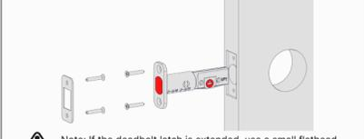
Note: If the deadbolt latch is extended, use a small flathead screwdriver to rotate slot until deadbolt latch is retracted.
