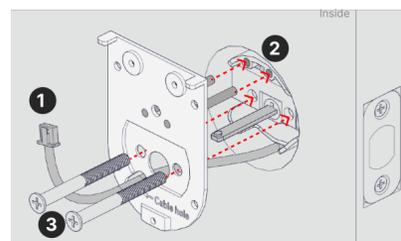
Refer to measurements B, C, and D on the Door Checker paper to select screws. Ensure that screws are secure enough, but DO NOT over tighten screws.
