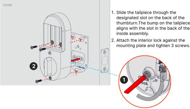
When fully tightened, lock should be flush to door.
